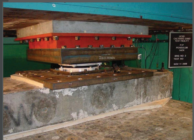
• Bi-directional type tests on a FIP-D isolator at the SRMD Test Facility at the University of California at San Diego, USA.
