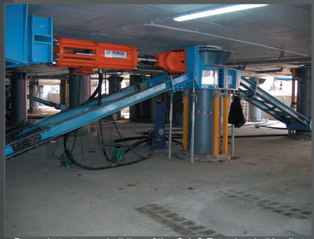
• Dynamic tests on a building of the C.A.S.E. project in L'Aquila (Italy) isolated with FIP-D devices.
